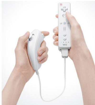
Figure 6.9: Nintendo Nunchuk, an additional hardware for Wii Remote, is equipped with a analog joystick, one button, and also with motion sensing [Nino7]
