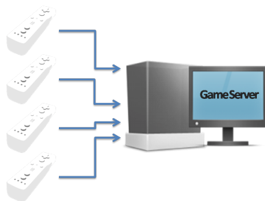
Figure 3.1: Using Bluetooth, one PC could connect up to four Wii Remotes
